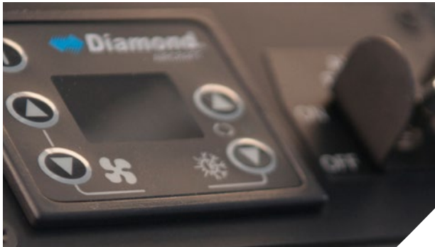
Air conditioning/RACC II system (powered by an additional alternator)
